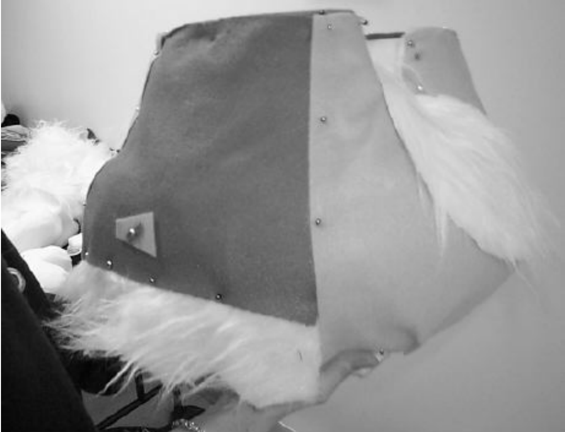
Figure 8: the foam shell (torso) of PETS 2
