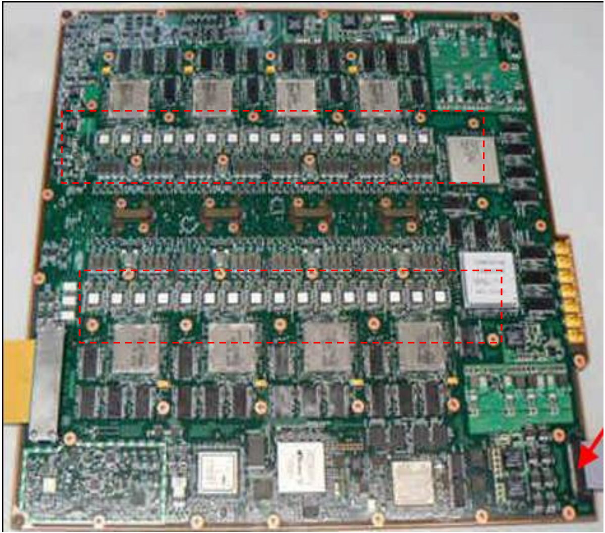
Figure 61 Product circuit board showing QFN's
