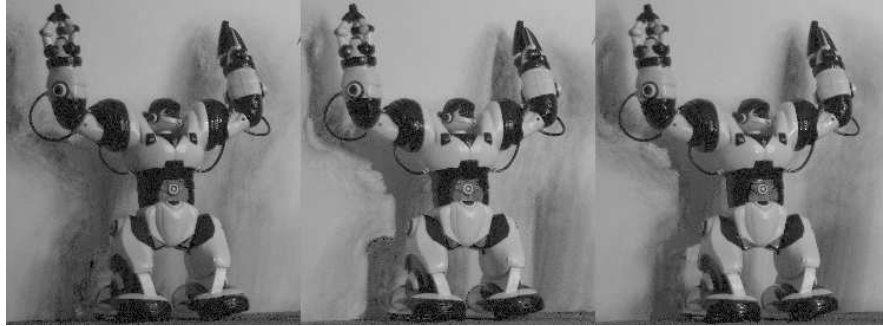
Figure 7.7: Reconstructed 16 \times 16 RF of a robot exhibiting both Lambert's and Specular shading from 128 compressive measurements using a HSS model. The top 64 Haar coefficients were chosen as the subspace B_p .
