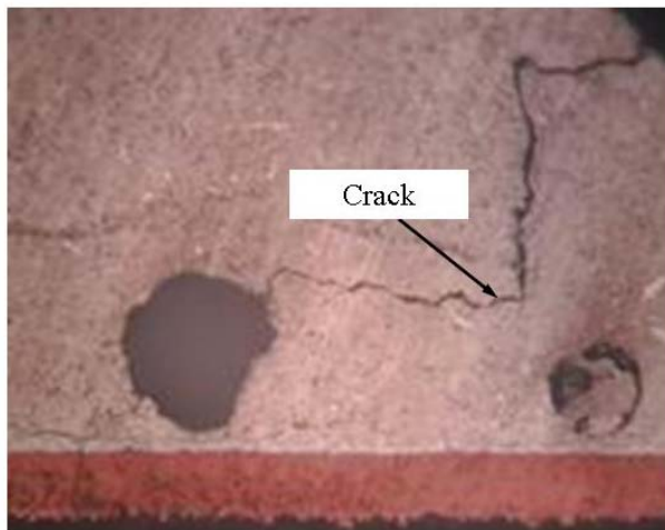
Figure 23: Crack in fillet of voided CLCC solder joint
