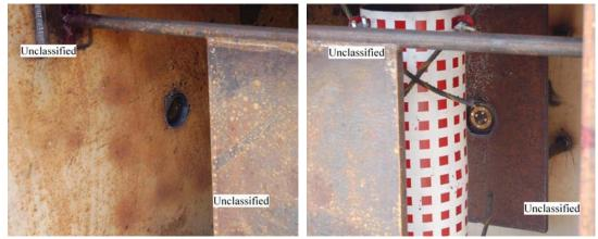
Figure 8.17. Confined blast post-test #2, pressure gage displacement.
