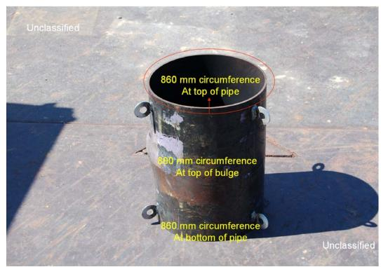
Figure 8.10. Confined blast post-test #1, view B of 15 in high cylinder deformation.
