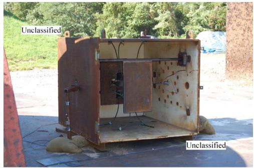
Figure 8.6. Confined blast post-test #1 view of interior.
