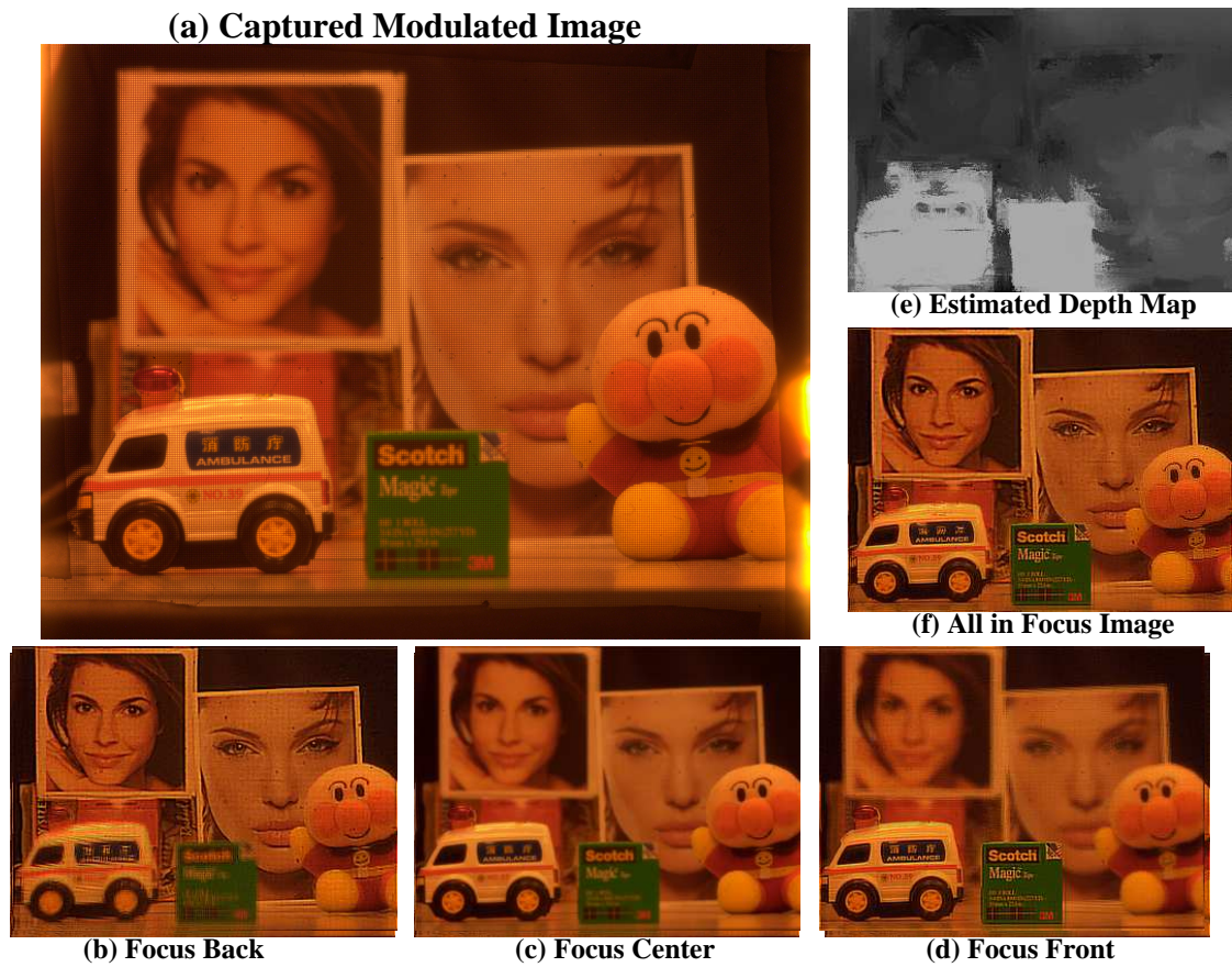
Figure 5.14: (a) Captured Modulated Image (b) Refocussed Image - Focus on back poster (c) Refocussed Image - Focus on doll (d) Refocussed Image - Focus on front Scotch box (e) Raw Depth labels quantized to 10 depth levels. (e) All in focus image.
