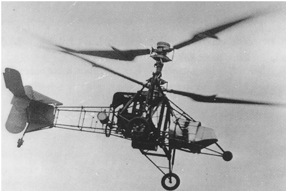
Fig. 1.3: The technically successful coaxial helicopter built by Breguet-Dorand in 1935 (Ref. 25).
