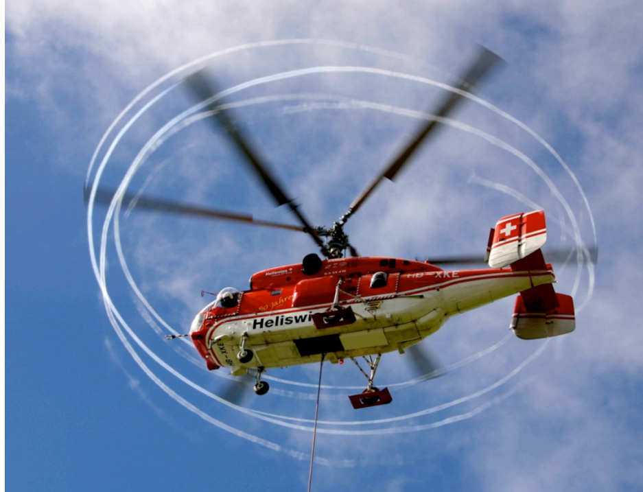
Fig. 1.5: Kamov Ka-32 coaxial helicopter, the rotor wake being rendered visible by natural condensation effect, and showing the interference of the flow between the two rotors (Ref. 25).
