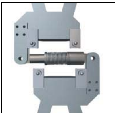
Figure 2.3: Illustration of a viscous damper implemented in the Millennium Bridge.
