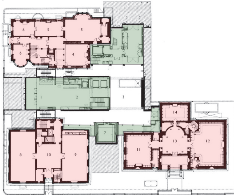
Figure 67. Grand Atrium as regularizing element: The grand atrium or “covered piazza” acts as the regularizing element to divide the connecting elements between the existing buildings (Author)
