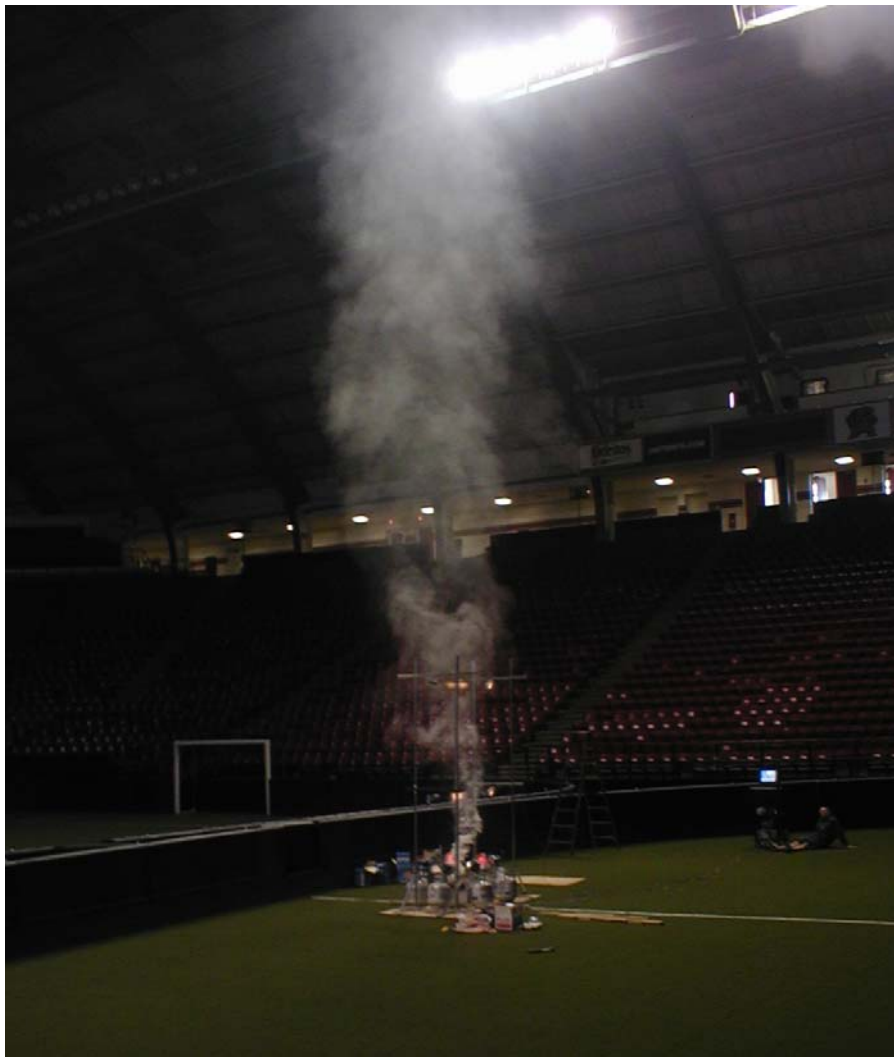
Figure 8 – Plume Tilt Depiction for 4 min Emitter at Low Lighting Level
