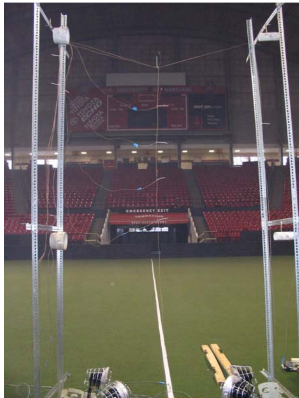
Figure 7 – ODM and Thermocouple Setup for Cole Field House
