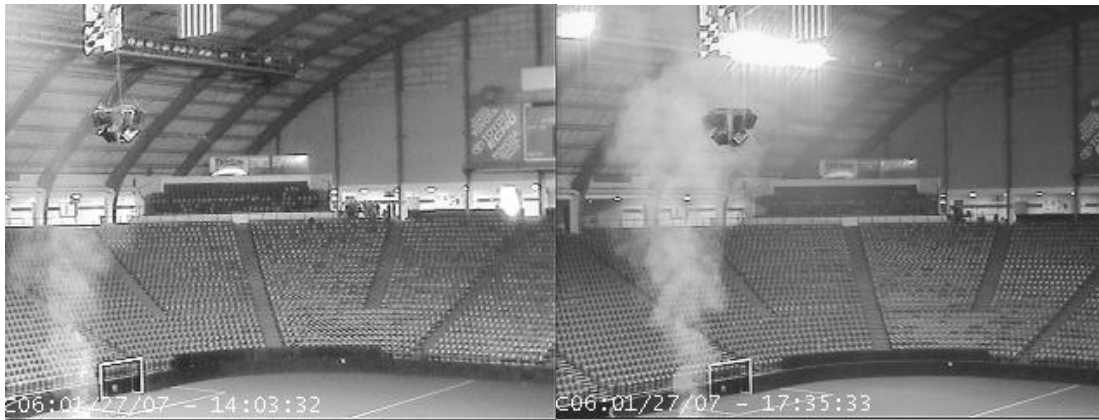
Figure 21 - Lighting Level Effect on Activation Time
