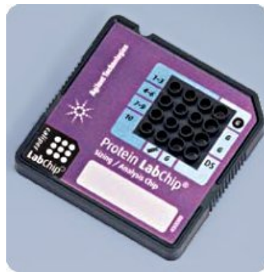
Figure 1.2: Agilent Technologies 2100 LabChip used for DNA, RNA, and protein analysis through electrophoresis.
