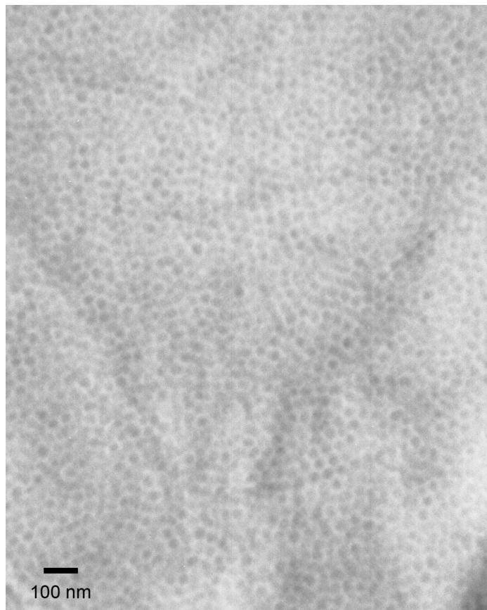
Figure 3.11: PS/P4VP microtomed along the constraint direction, showing the cylinder ends. Contrast comes from nickel in the P4VP block.
