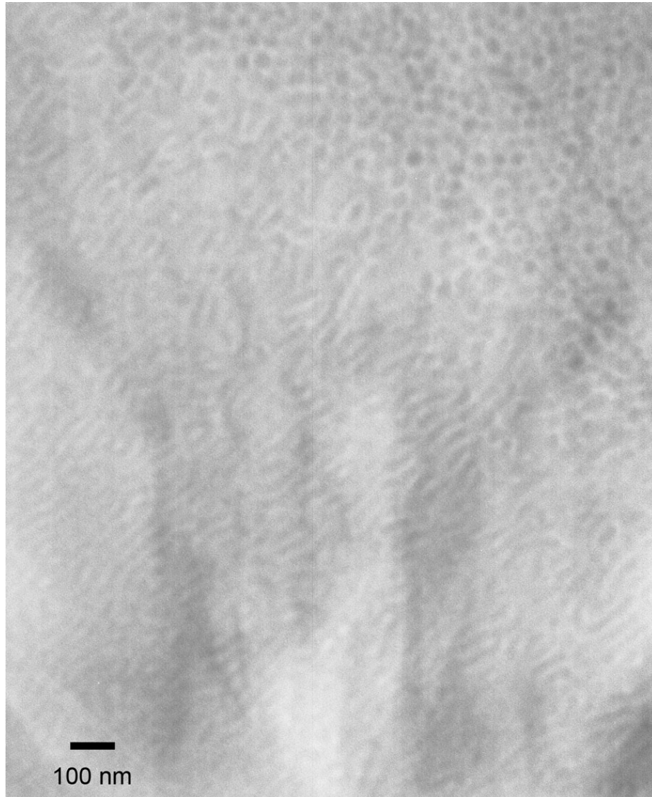
Figure 3.3: TEM micrograph showing both the sides and the ends of the cylindrical microstructure resulting from PS/P4VP-Ni film formation from static casting from 8.5 % tetrahydrofuran and 91.5 % chloroform. The \text{Ni}^{2+} ion in the P4VP block provides contrast.
