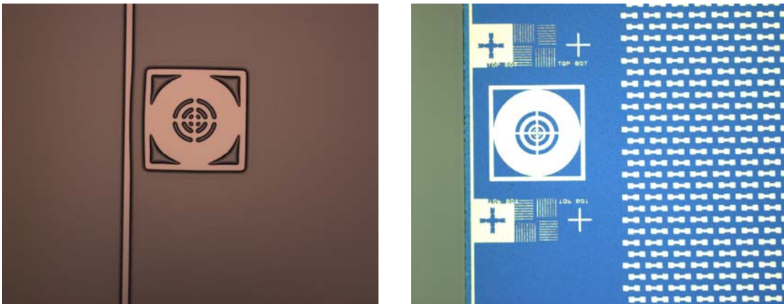
Fig 3.6 Alignment marks in acrylic (left) and metallized die test pattern (right). Slight heat deformation visible in acrylic. The target patten is 220\mu\text{m} in diameter.
