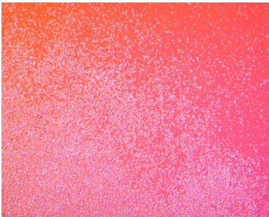
Fig 2.6. Particle agglomeration on wafer surface as viewed through a Nomarsky filter. 50x magnification.
