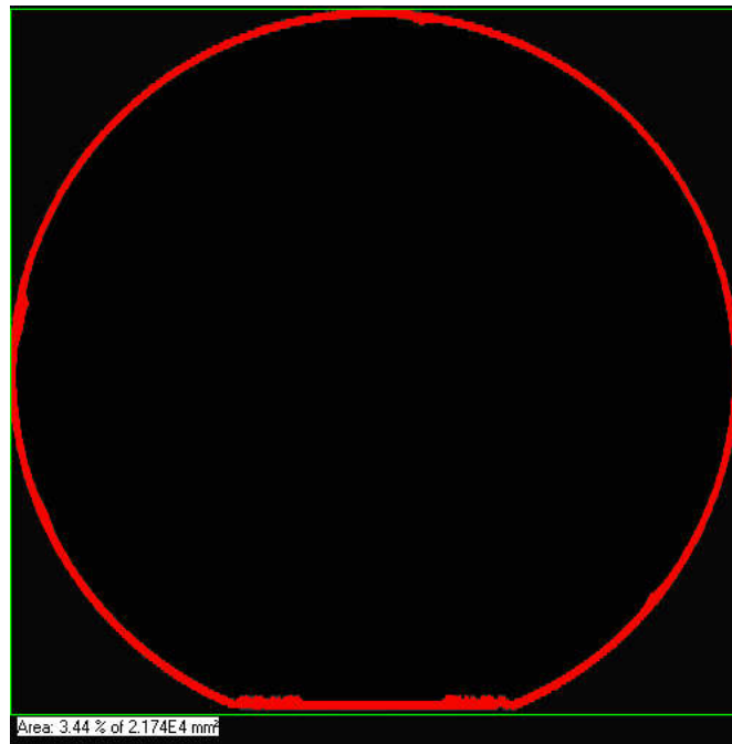
Fig. 2.9. Void free bond. Un-bonded areas appear in red. Image taken by SAM.
