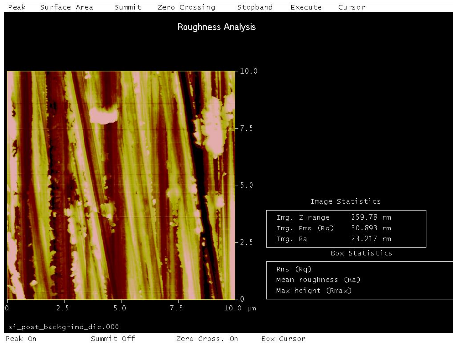
Fig 2.2. Surface roughness after mechanical grinding
