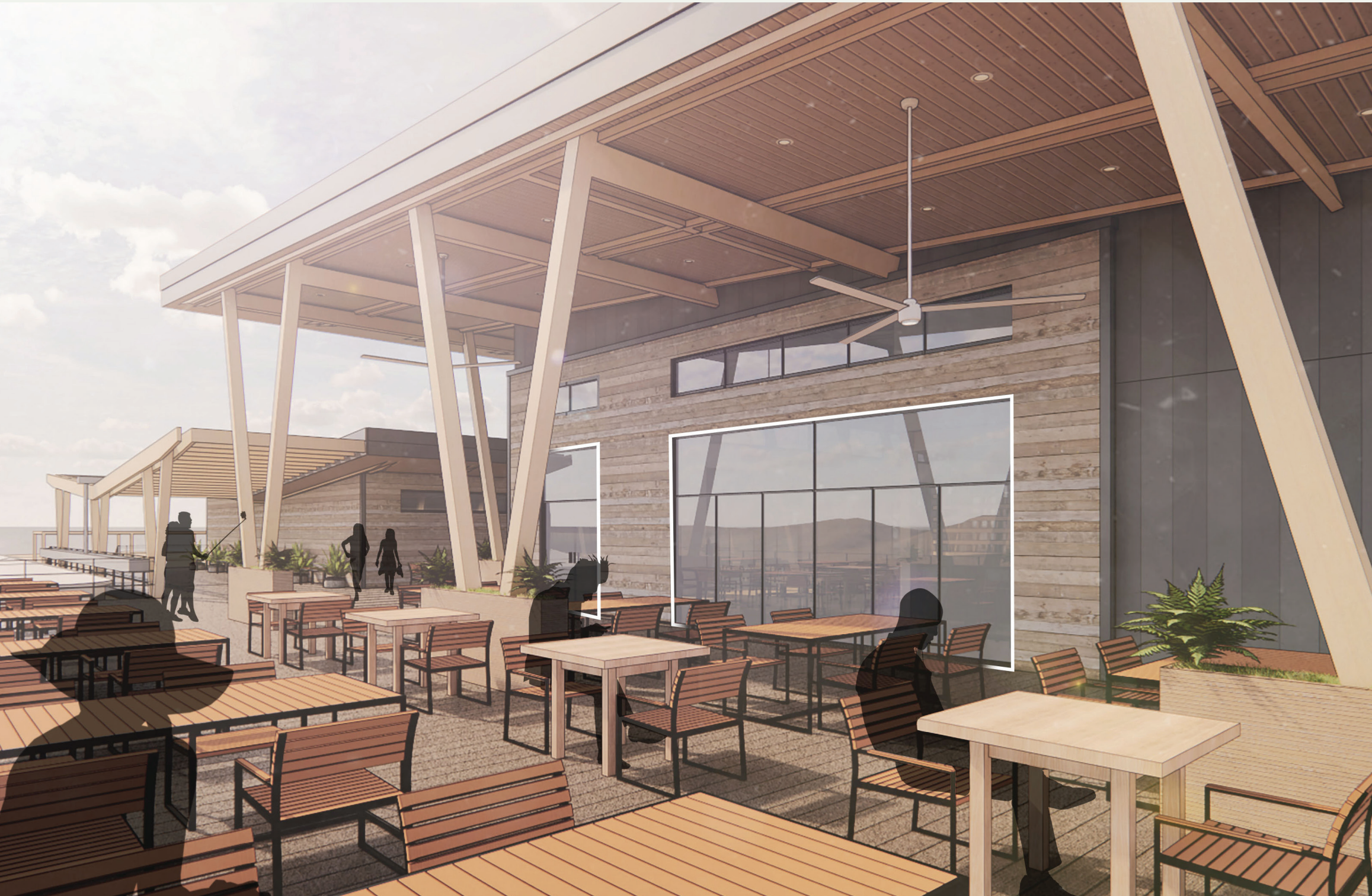
THE BUILDINGS CAPTURE SEASONAL WINDS TO ASSIST IN COOLING AND VENTILATION. NATURAL VENTILATION IS COMPLEMENTED WITH CEILING FANS.
