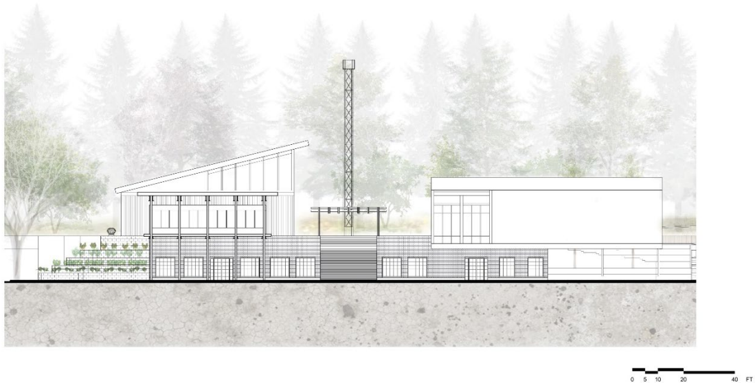
Figure 92: West elevation showing entry gate threshold to upper terraces and relocated signal tower.
