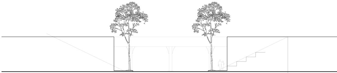
Figure 103: Previous section study. Diagonal line is the noon sun angle for the winter solstice in Chicago.
