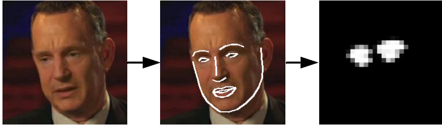
Figure 6.2: Mask generation pipeline. First parts are detected using dlib, then the masks are created from the convex hulls of the detected regions. Finally, masks are post-processed with morphological dilations and gaussian blur.
