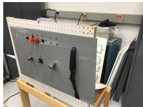
Fig. 4 Task board. Top row, from left to right: push button, switch with switch guard (flip up), switch with switch guard (flip down), push button, switch without switch guard (x2). Bottom row from left to right: electrical connector, knob, buckle.
