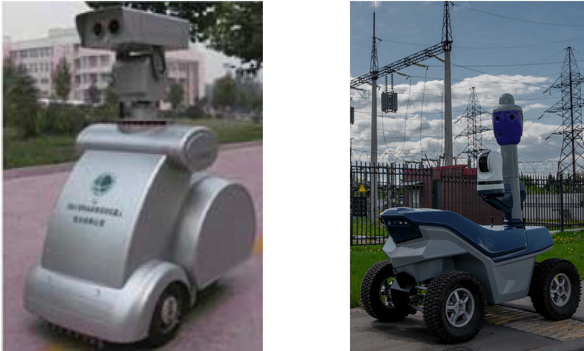
Fig. 7 Examples of maintenance inspection robots: SmartGuard Robot (left) [27] and Electrical Substation Inspection Robot (right) [28].
