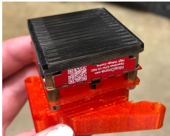
Fig. 24 NicaDrone EPM end effector in a 3D printed mount for the Baxter robot.
