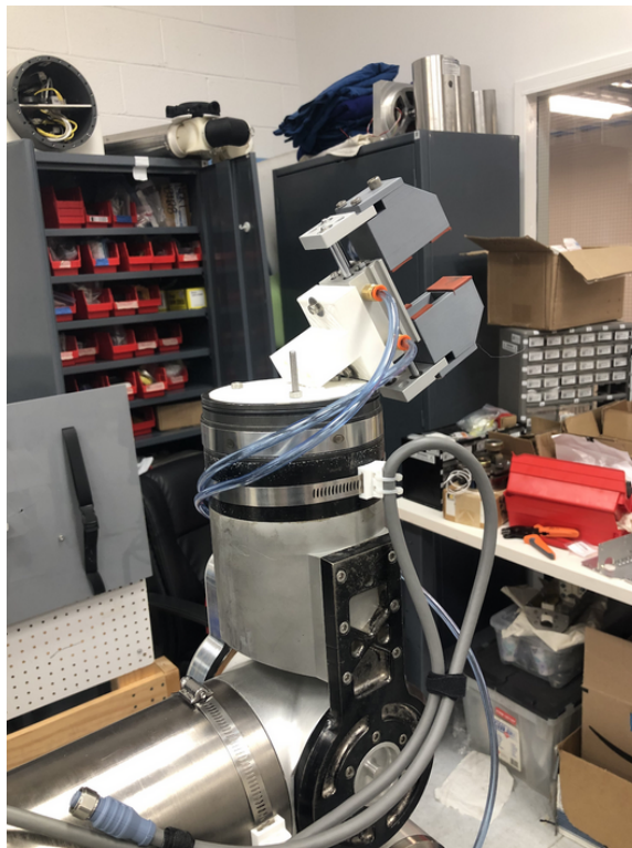
Fig. 22 The pneumatic gripper mount broke, as it sheared along the bottom of the mounting, between the circular plate and the shaft. A redesign of the mounting system to be mechanically stronger was needed.
