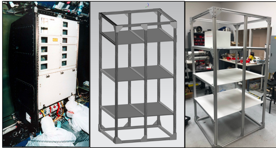
Fig. 25 ISPR being installed in the ISS Destiny Module (left) [46], CAD model of rack mock-up (center), constructed mock-up of ISPR used for testing (right).
