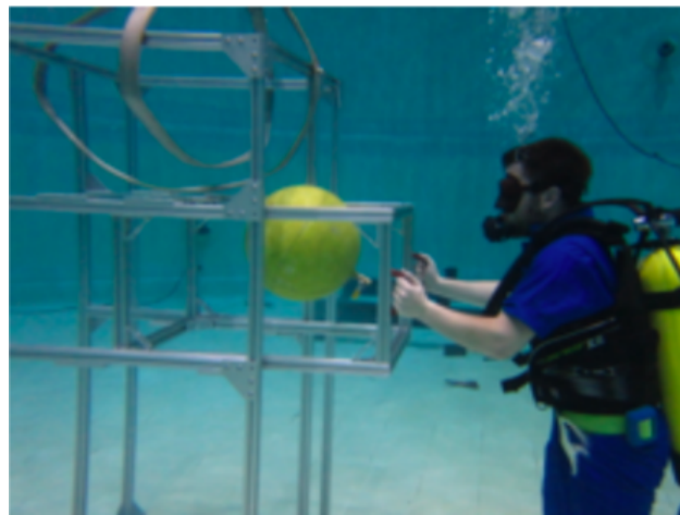
Fig. 5 Testing functionality of rack slides in prototype Oxygen Generator Assembly mock-up.
