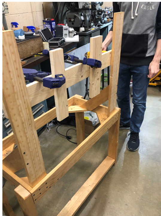
Fig. 16 Additional wooden supports added to the updated taskboard to prevent flexing during testing.
