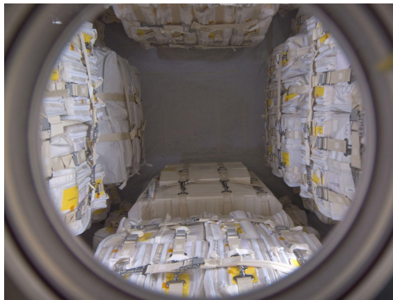
Fig. 8 JAXA H-II Transfer vehicle docked to ISS Harmony module showing vast number of CTBs [30].
