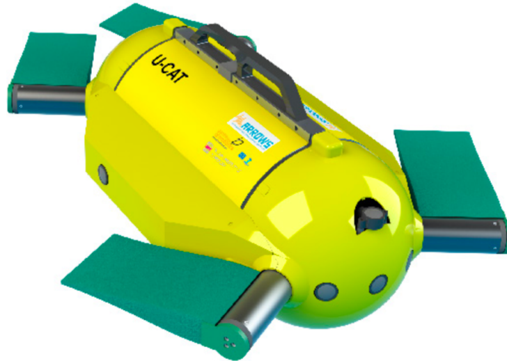
Fig. 40 Aquatic robot designed for looking through dangerous underwater zones that shouldn't be entered by humans, such as complex tunnels, ship wrecks, and severely damaged underwater pipelines. It can be used to clean important artifacts found underwater, and could possibly be improved with the team's research on the use of different end effectors for varying tasks [59].
