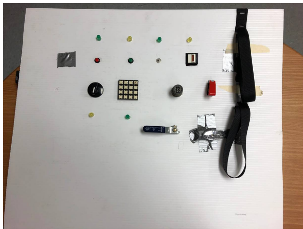
Fig. 2 Taskboard Layout: Pictured are buttons, switches, knobs, valves, an electrical connector, and a buckle.
