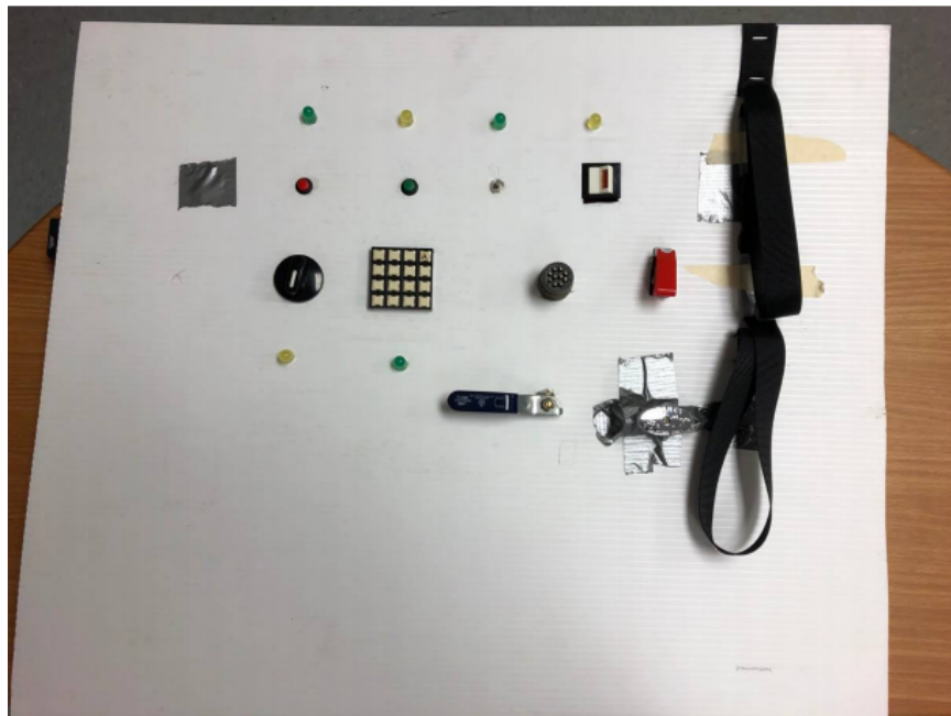
Fig. 14 Preliminary taskboard with low fidelity and high fidelity tasks, such as switches, knobs, and buckles, wired to LEDs.
