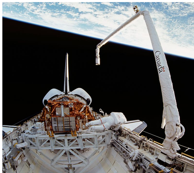
Fig. 3 Canadarm on orbit as a part of the Shuttle's Remote Manipulator System [15].
