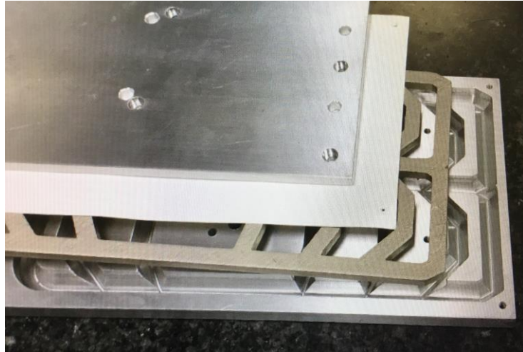
Figure 3.12: Exploded view of single phase microchannel liquid cooled cold plate. Thermal Stack includes: branched out heat pipe, interface material, metal plate and clamping mechanism
