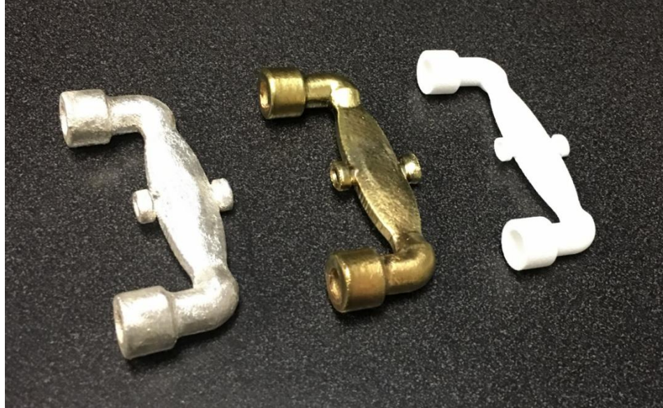
Figure 5.27: Fabricated elliptic coupling with AM SLS technology: (left to right) 1). Electroless .1" silver plated nylon 6,6 . 2) Electroforming .1" copper with gold finish nylon 6,6 and 3). Bare nylon 6,6. (lengths of coupling are 50,20 and 5mm along flow, electrode and magnetic flux directions respectively)
