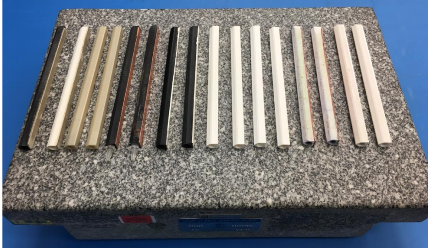
Figure 4.10: Set of LM compatible tubes. The core material of the tubes is either CNC machined solid BN ceramic (white), or FDMed Ultem polymeric (black or gold color). Electroplating of silver or copper applied for fusion purposes during in-situ SLM AM process as next embedding step of fabricating cold plate.
