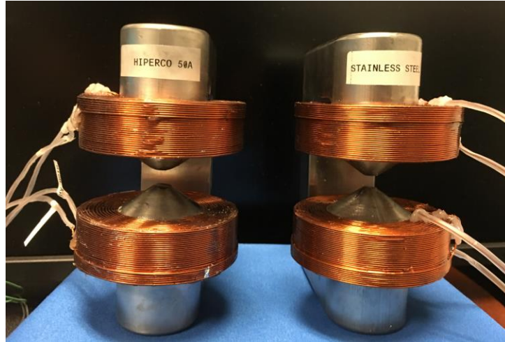
Figure 5.16: MHD pump electromagnets with two magnetic materials for C-shaped core (hiperco50A vs magnetic stainless steel)
