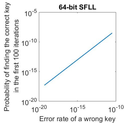
Figure 5.2: The positive correlation between the error rate of wrong keys and the probability that SAT finds the correct key in certain iterations
