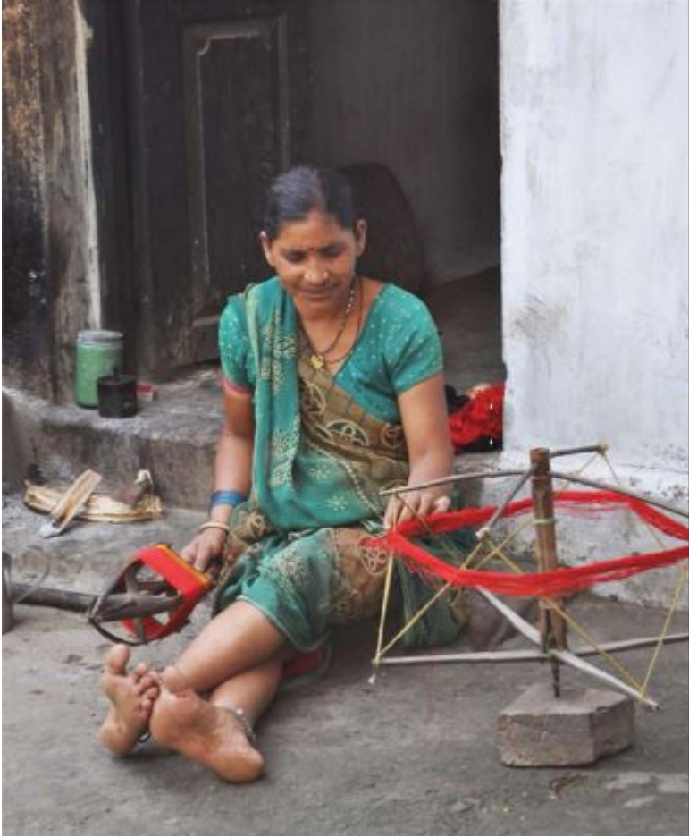
Figure 21 The home made equipment used for winding
