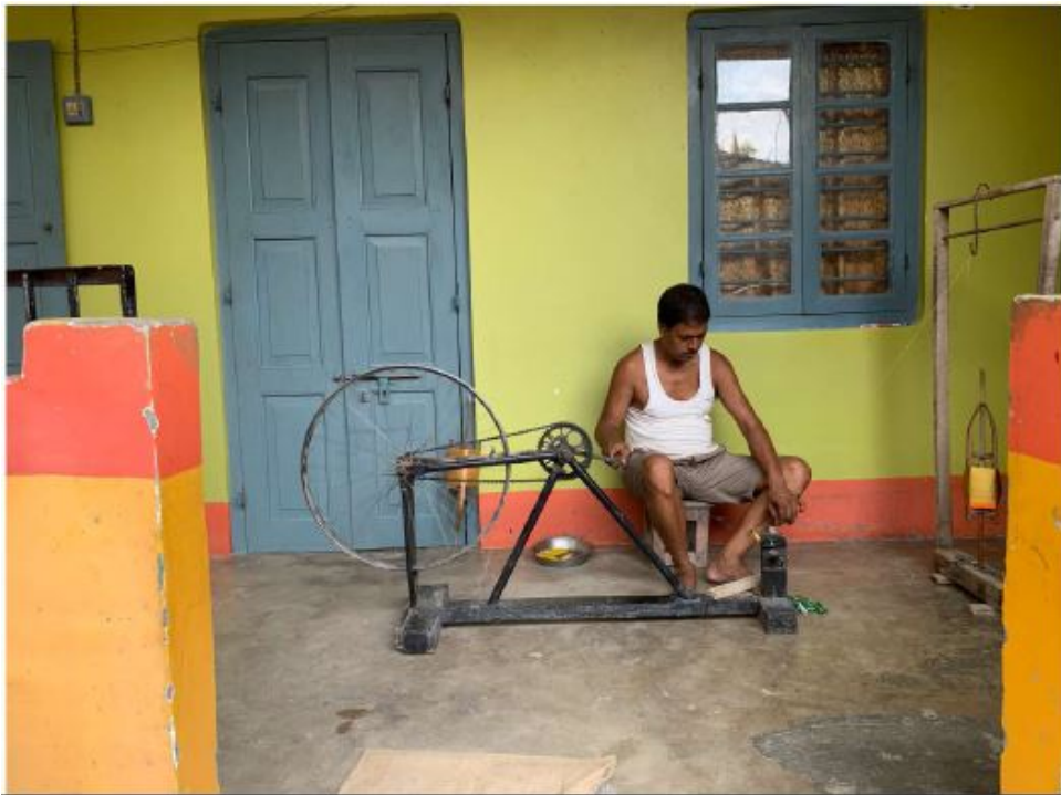
Figure 14 The current means of people to form a hand spinner from a bicycle
