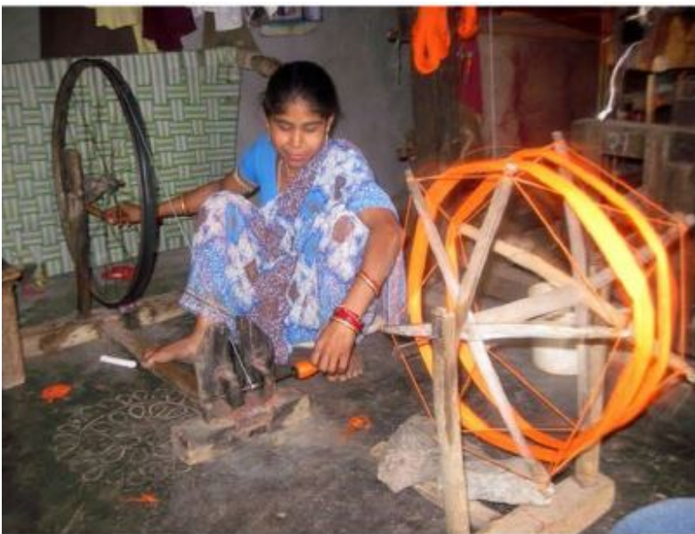
Figure 34 The weft winding done by a charkha
