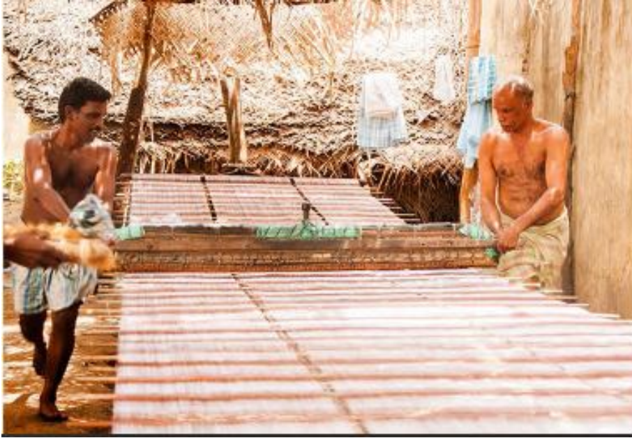
Figure 25 street sizing done in a backyard of a workshop
