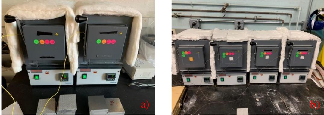
**Figure 6.** Thermo Scientific Thermolyne furnace FB1400 at UMD. (a) Furnace 1 (F1) and Furnace 2 (F2) from left to right and (b) Furnace 3 to Furnace 6 (F3 to F6) from right to left.
