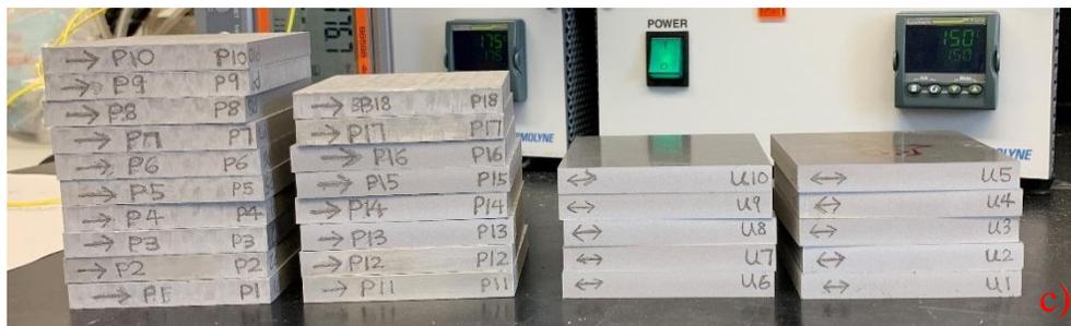
**Figure 4.** (a) As-received laser shock peened AA5083-H116 samples, (b) As-received no laser shock peened AA5083-H116 samples, and (c) Total 28 AA5083-H116 samples with 18 laser shock peened samples (left) and 10 no laser shock peened samples (right).
