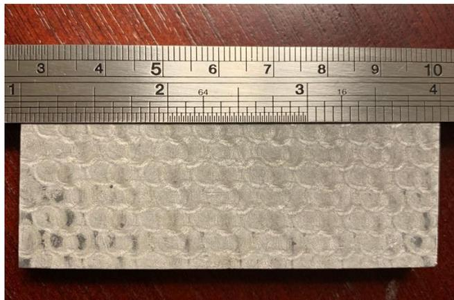
**Figure 22.** The array of circles appears on the laser shock peened sample surface. The diameter of each circle is about 6.35mm (0.25in).
