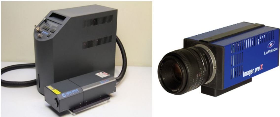
Figure 3.3: Optics. Left: New Wave Nd:YAG SOLO II- PIV/PLIF 532 nm wavelength, 15 Hz pulsed laser (source: New Wave Research [68]); right: LaVision ProX 4M pixel CCD camera (source: LaVision [67]).
