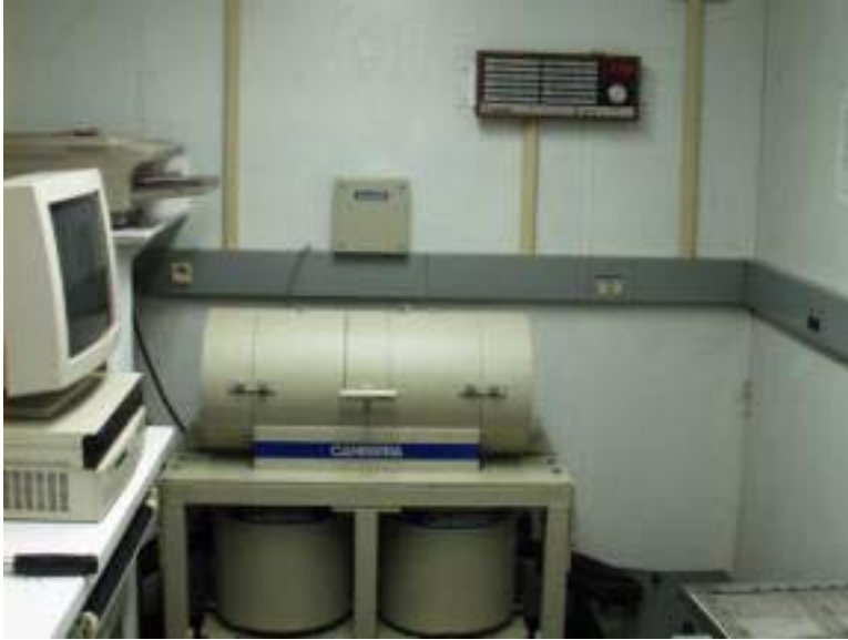
Figure 22: CA002 Detection System with Low Background Cover Closed
