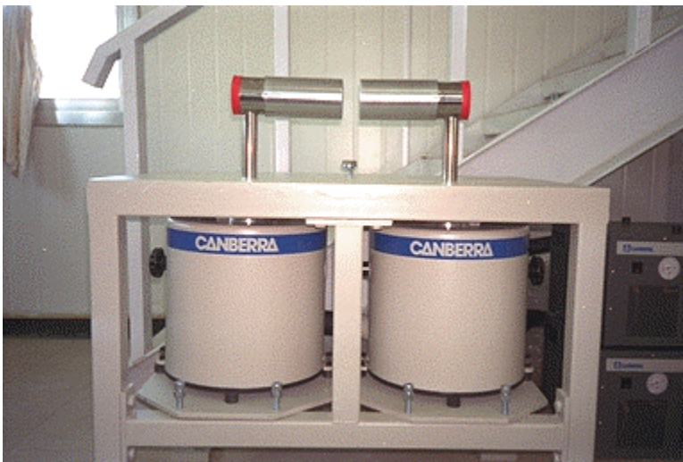
Figure 23: Representative Example of Detection System Uncovered
