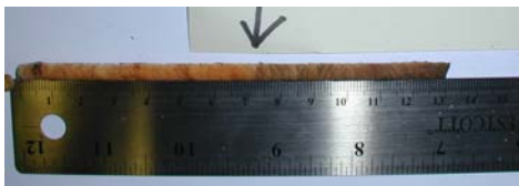
Figure 6 Tree core showing obvious heartwood/sapwood boundary. Color differences due to tylose blockage in inactive heartwood (to the right).
