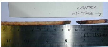
Figure 7 Tree core exhibiting severe decay.
