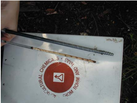
Figure 5 Tree increment borer. Upper drill bit is used to penetrate tree and lower extractor sleeve is used to retrieve a 5-mm diameter core.
