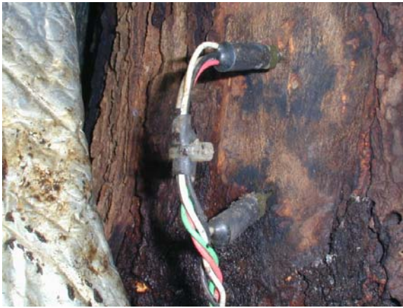
Figure 12 One set of thermal dissipation probes.
