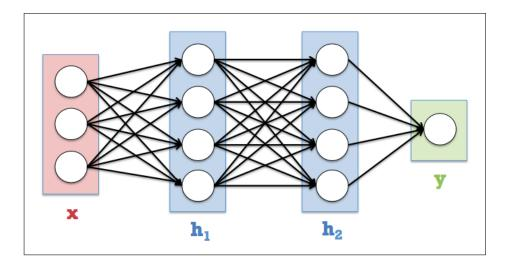
Figure 2.6: A fully connected feedforward neural network with an input layer, two hidden layers (with four hidden units each) and an output layer.
