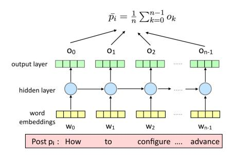
Figure 4.6: Our LSTM architecture on a post  $p_i$ . The input layer consists of pretrained word embeddings of the words in the post which is fed into a single hidden layer. The output  $o_k$  of each of the hidden states is averaged together to get our neural representation  $\bar{p}_i$
