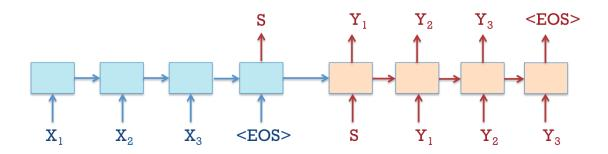
Figure 2.8: Sequence-to-sequence learning model which takes in an input sequence and generates an output sequence one word at a time.
