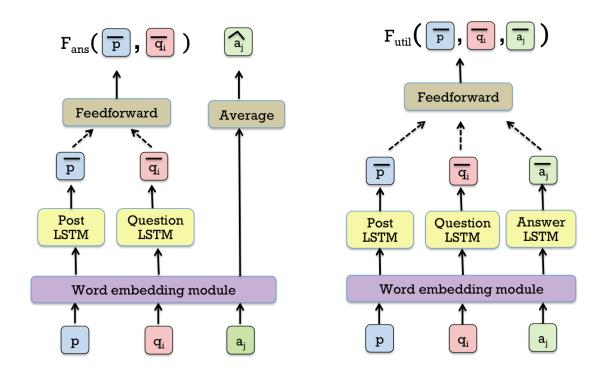
Figure 4.5: Left:  $F_{ans}$  computed using a feedfoward neural network over post LSTM  $\bar{p}$  and question LSTM  $\bar{q}$  representations and  $\hat{a}$  computed using average word embeddings over words in the answer. Right:  $F_{util}$  computed using a feedforward neural network over post LSTM  $\bar{p}$ , question LSTM  $\bar{q}$  and answer LSTM  $\bar{a}$  representations. estimate the probability of answers.
