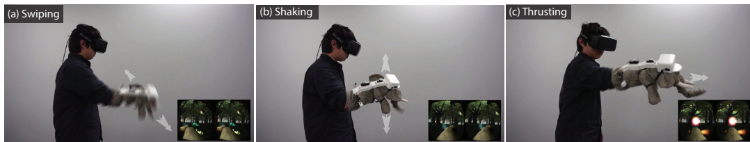
Figure 5.4: This figure shows three gestures we designed to control the virtual character: (a) swiping from left to right triggers the character to swing the nose and blow wind, (b) shaking up and down triggers the character to splash water, and (c) thrusting from inward to outward triggers the character to howl, trample on the ground and throw fireballs. A video demonstration is included at www.vrsurus.com .
