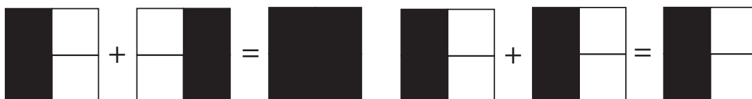
(b) Revealing a black or (noisy) white block using two shares of images
