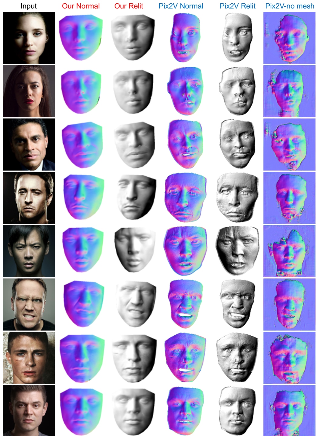
Figure 10-5: SfSNet vs Pix2Vertex [133] on images selected by us with non-ambient illumination and expression. ‘Relit’ images are generated by directional lighting and uniform albedo selected to highlight the quality of the reconstructed normals. (Best viewed in color)
