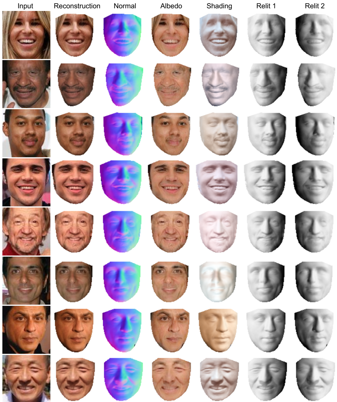
Figure 10-3: Results of SfSNet on CelebA. ‘Relit’ images are generated by directional lighting and uniform albedo to highlight the quality of the reconstructed normals. (Best viewed in color)
