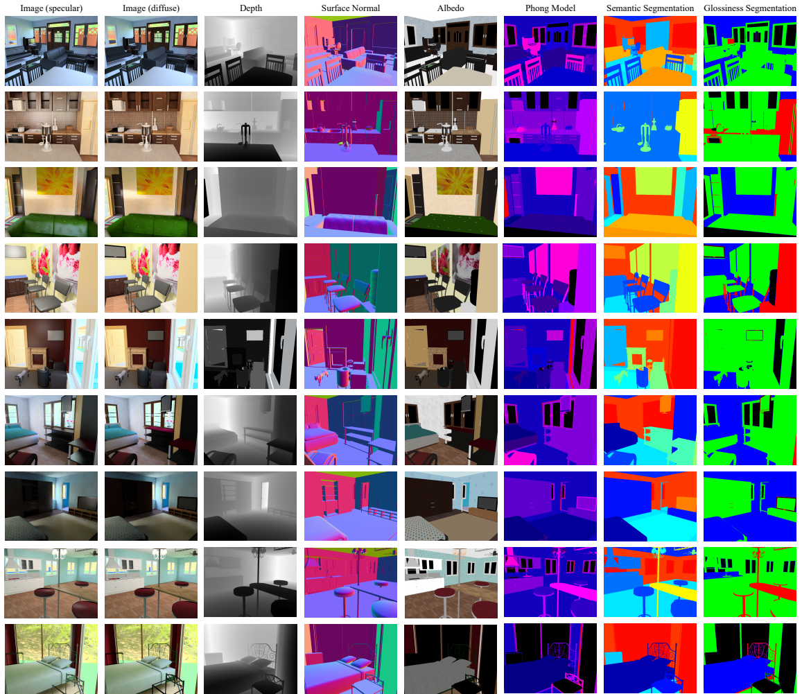
Figure 10-16: Our SUNCG-PBR Dataset. We provide 235,893 images of a scene assuming specular and diffuse reflectance along with ground truth depth, surface normals, albedo, Phong model parameters, semantic segmentation and glossiness segmentation.
