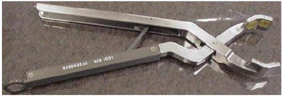
Figure 5.3 CATS High Torque (HT) Connector Tool
