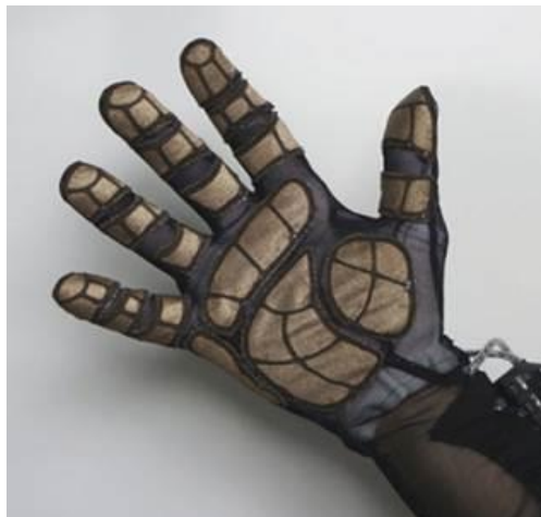
Figure 1.3: A sensing glove made of conductive fabrics [31].
