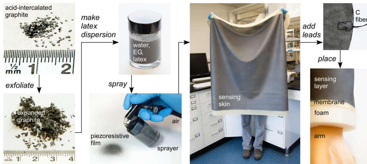
Figure 4.1: Formation of the sensing skin. Acid-intercalated graphite is expanded, the layers are separated in an aqueous solution (not shown), and latex is added to form a paintable dispersion that is spray-coated onto a rubber membrane to form an EG/latex piezoresistive sensing skin. Large areas are possible. Electrical connections are made with carbon fiber bundles using additional EG/latex as an adhesive. The skin can be placed over a layer of foam to form a skin+foam stratum.
