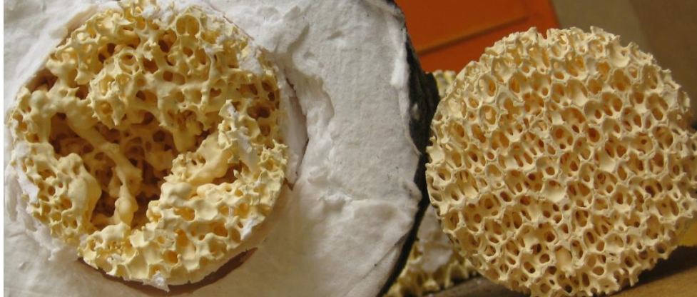
Figure 2-5. Damaged and undamaged ceramic foam[9]
