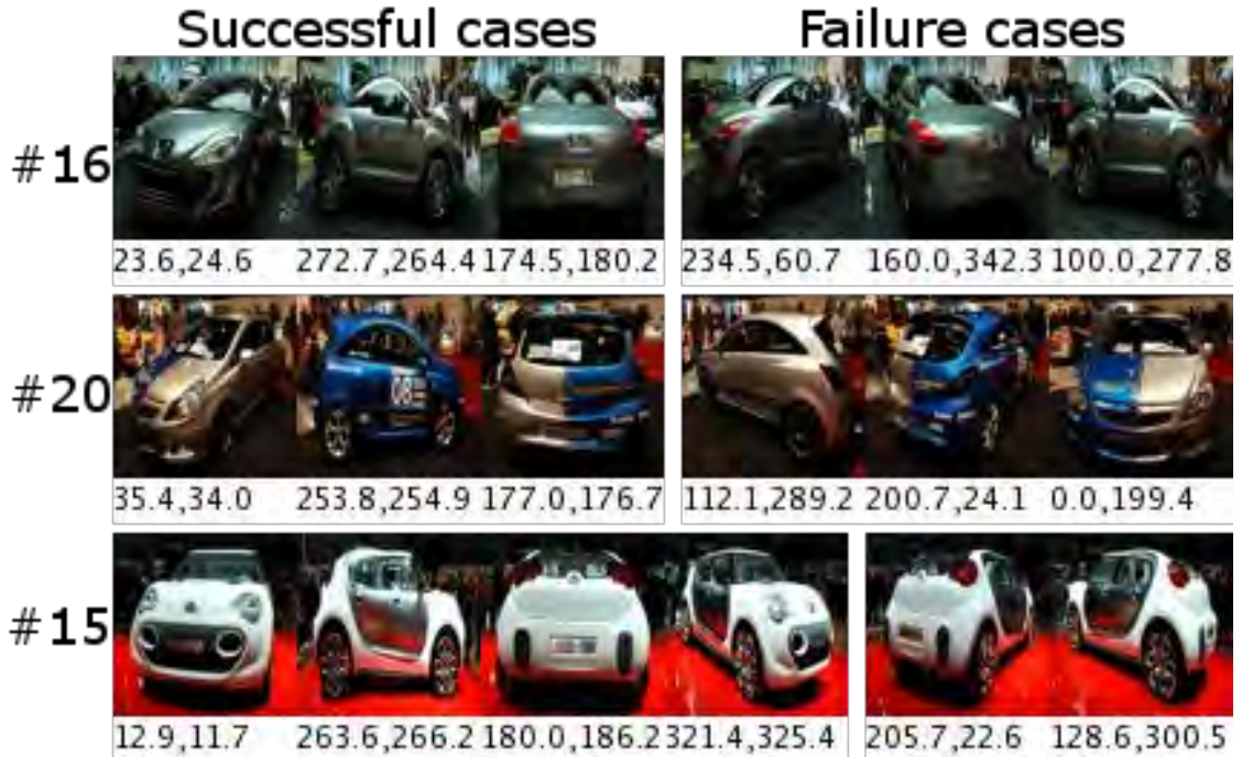
Figure 3.7: Representative results from the worst three sequences in the testing set. The numbers under each image are the ground truth direction (left) and the estimated direction (right). Most of the failure cases are due to the flipping error.
