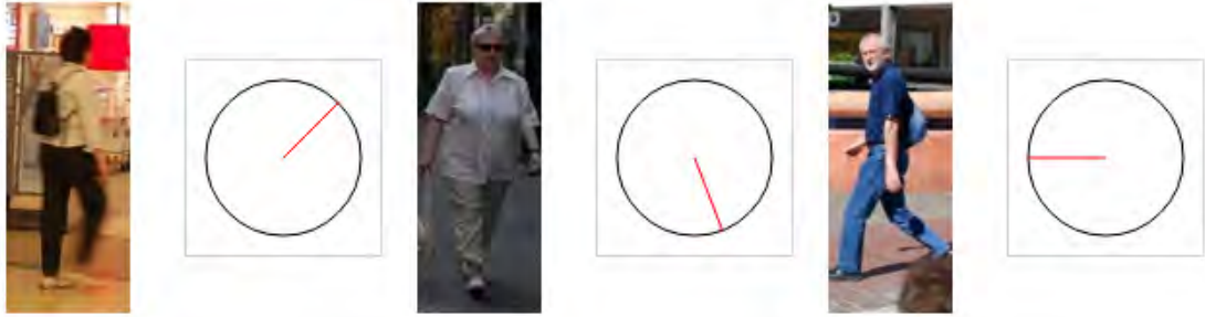
Figure 3.1: User interface for the continuous orientation annotation. Each annotator is requested to specify the body orientation of pedestrians by moving a line segment in a circle.
