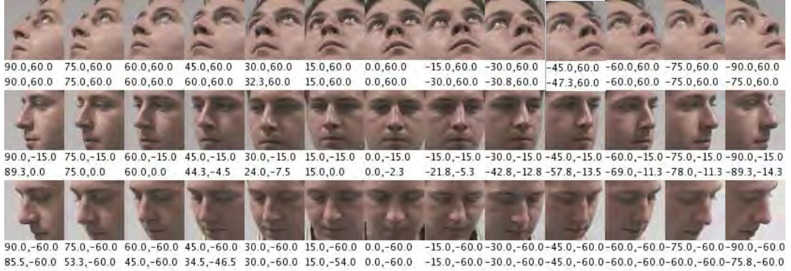
Figure 3.4: Some estimation results of the second sequence of person 13. The top numbers are the ground truth yaw and pitch and the bottom numbers are the estimated yaw and pitch.
