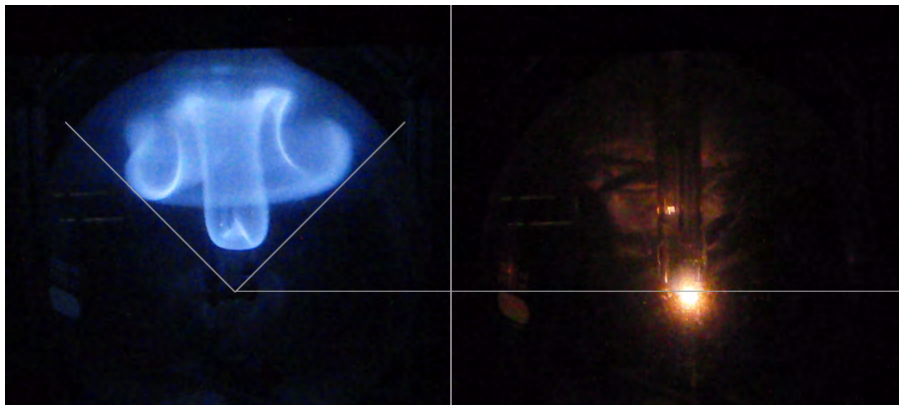
Figure 14: An example of a “Flammable” result with the stopper at 14.8%
