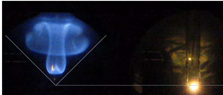
Figure 13: An example of a “Nonflammable” result with the stopper at 14.7%
