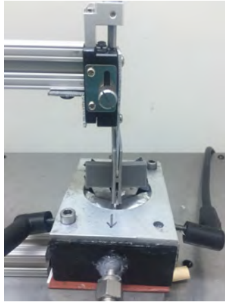
Figure 8: Front View of a Successful Burst
