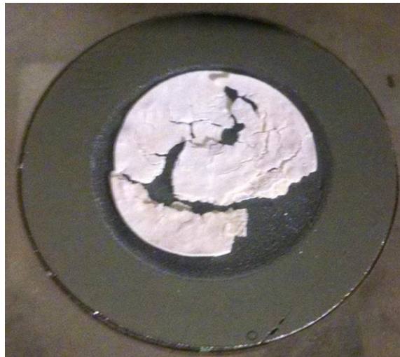
Figure 66. Photograph of sintered trilayer cell.
