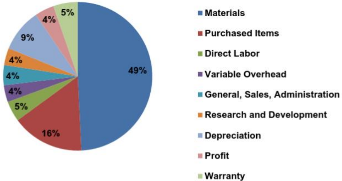
Figure 8. BatPaC model for lithium ion battery cost breakdown from ref. 32.
