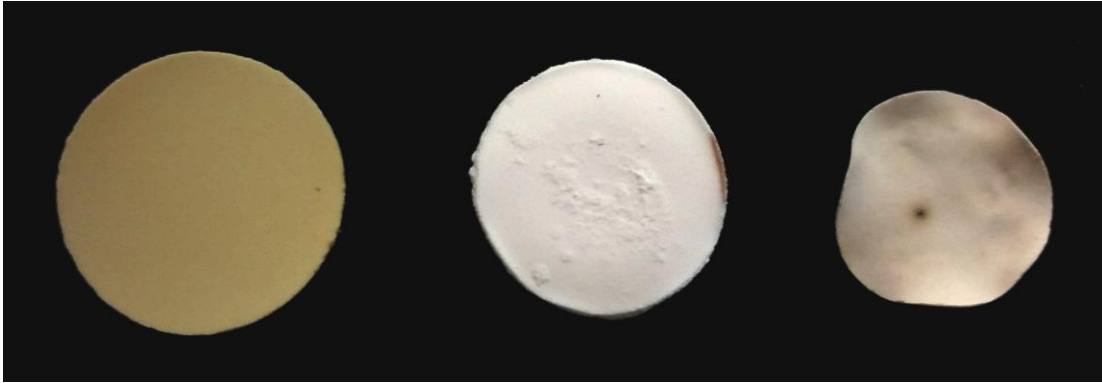
Figure 60. Photograph of three layer laminated garnet tape before pre-sintering (left), after pre-sintering exposed and sintering in argon at 1100 °C for 5 hours with powderbed (middle), without powderbed(right). The sintered samples shown were next to each other in the same crucible during sintering.
