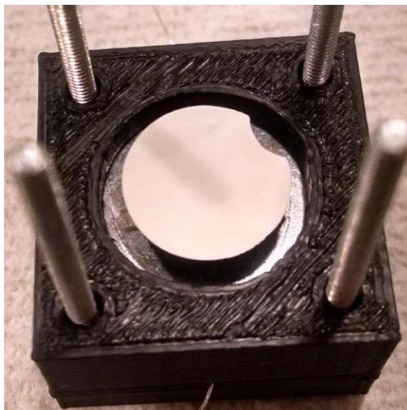
Figure 75. Photograph of intact triple layer garnet after nondestructive impedance testing.
