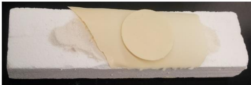
Figure 48. Photograph of the garnet disc ready for sintering on a porous Al 2 O 3 plate, covered in garnet powder, sacrificial garnet tape, and the target tape disc.
