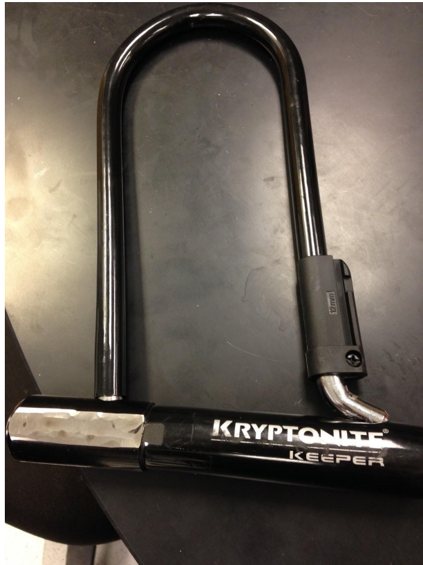
Figure 16. Kryptonite Keeper 12 U-lock after tension testing. The lock failed at the interface between the shackle's bent foot and the crossbar.
