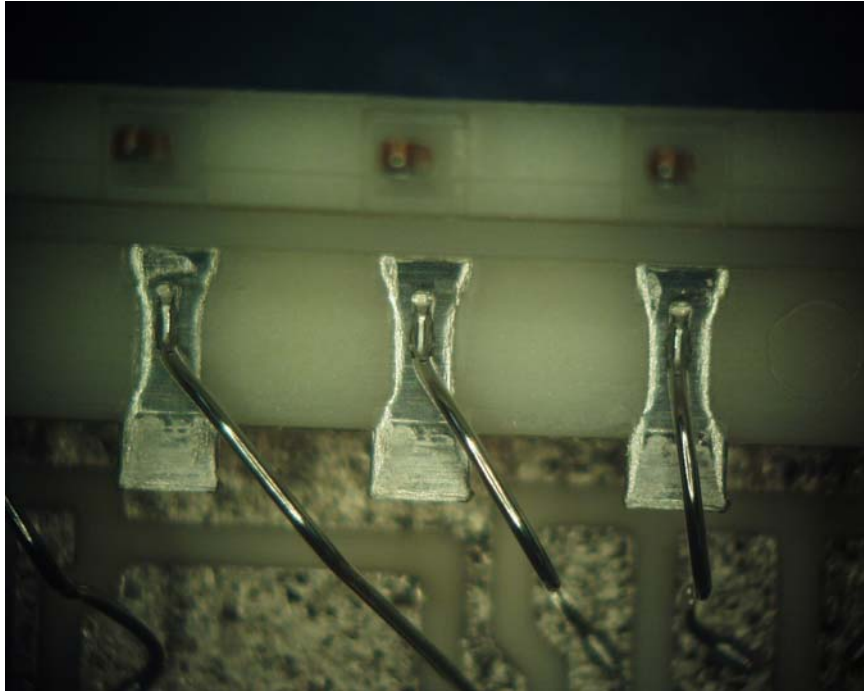
Figure 1-11 Wires bonded with twist in hybrid power modules
