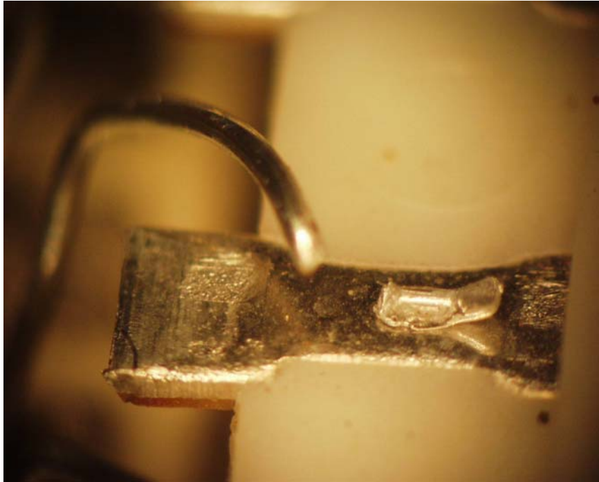
Figure 1-15 Failure of wire at the heel for a twisted wire
