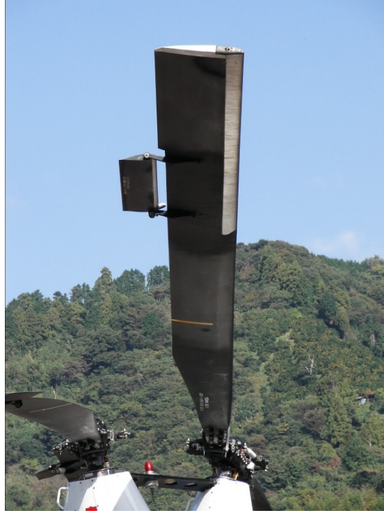
Figure 1.11: Servo - flap on a Kaman K-MAX rotor [35].
