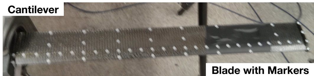
Figure 6.21: Blade with Vicon markers.
