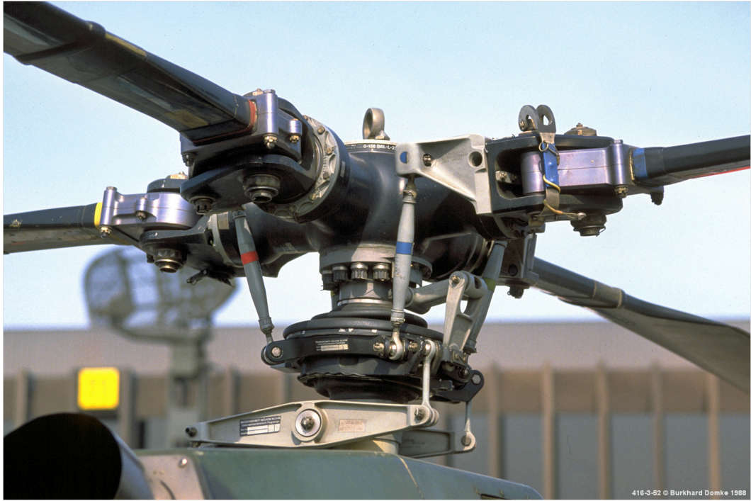
Figure 1.6: Close-up view of Bo 105 hingeless rotor system [12].
