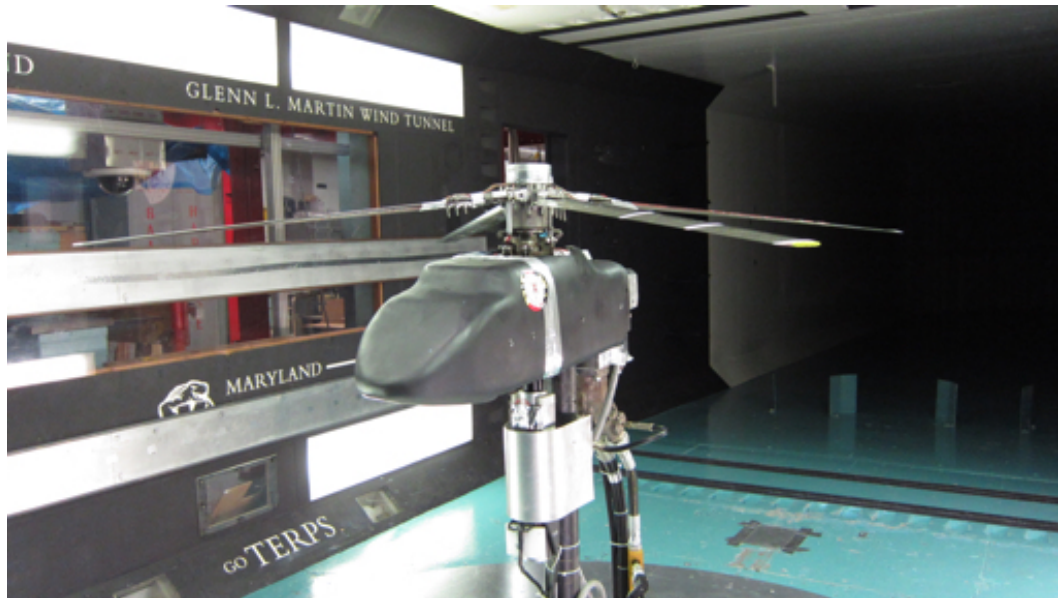
Figure 2.79: Rotor test stand installed in Glenn L. Martin wind tunnel.
