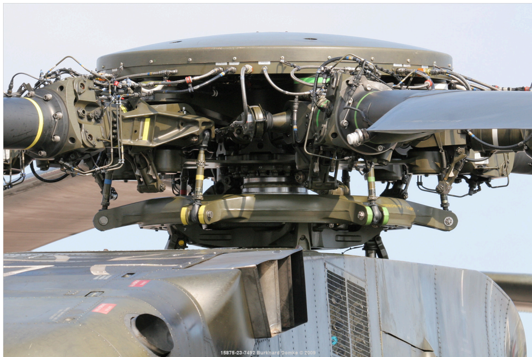
Figure 1.5: Close-up view of CH 53G fully-articulated rotor system [11].
