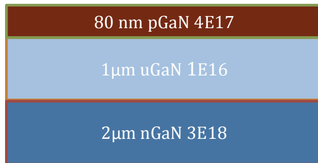
Figure 3-1 Film structure of the GaN sample
