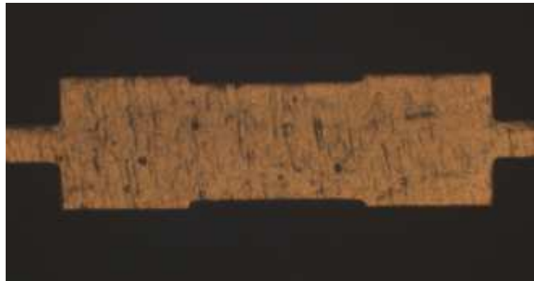
Figure 33: Shorted solder pads
