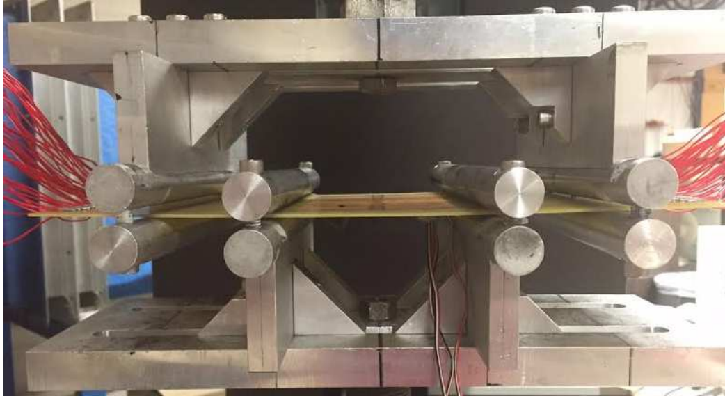
Figure 36: Fully reversible four-point bend test fixture
