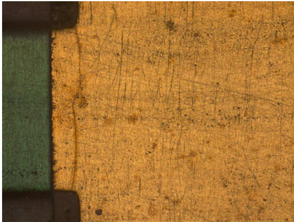
Figure 50: Trace cracking in solder masked boards
