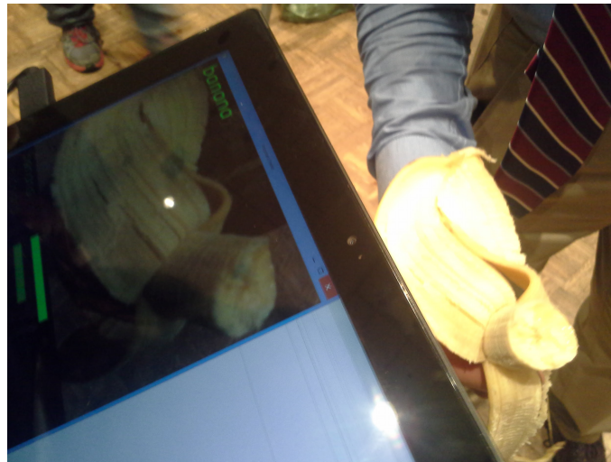
Figure 8.1: The device identifying a banana using the kernel descriptors algorithm
