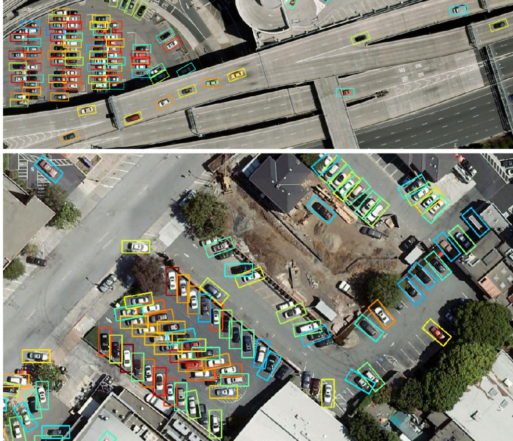
Figure 4.6: Sample vehicle detections the Google 90° dataset. Color represents the confidence of detection, red (high confidence) and blue (low confidence) being the two extremes. ©Google.
