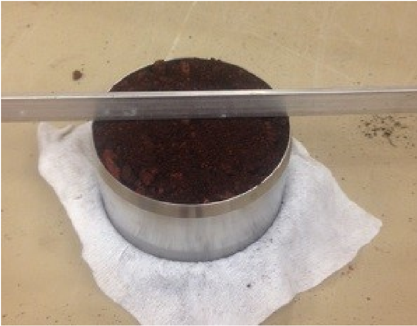
Fig. 3.4. Photograph illustrating an amended packing procedure for HYPROP® cores for use with coarse substrates.
