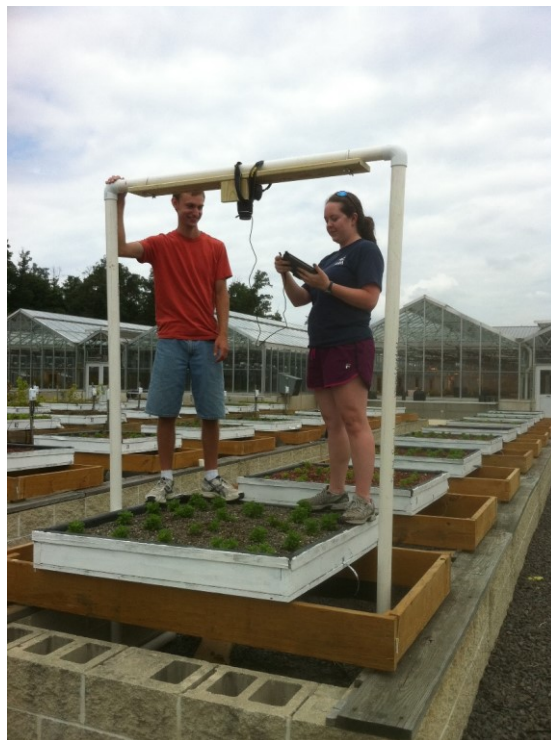
Fig. 5.7. Photograph illustrating overhead picture-taking for canopy coverage analysis. October 2013.
