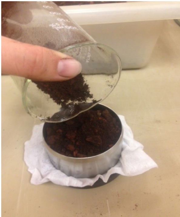
Fig. 3.2. Photograph illustrating an amended packing procedure for HYPROP ® cores for use with coarse substrates.
