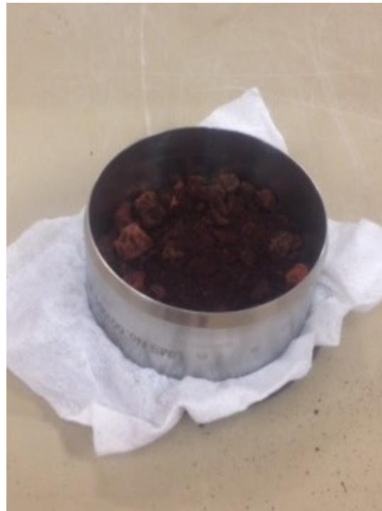
Fig. 3.3. Photograph illustrating an amended packing procedure for HYPROP ® cores for use with coarse substrates.
