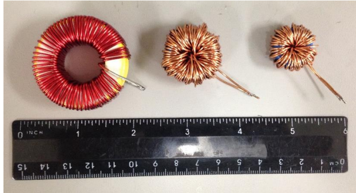
Fig. 7.2. PFC inductors switched at 100 kHz, 500 kHz, and 1 MHz (from the left to the right).
