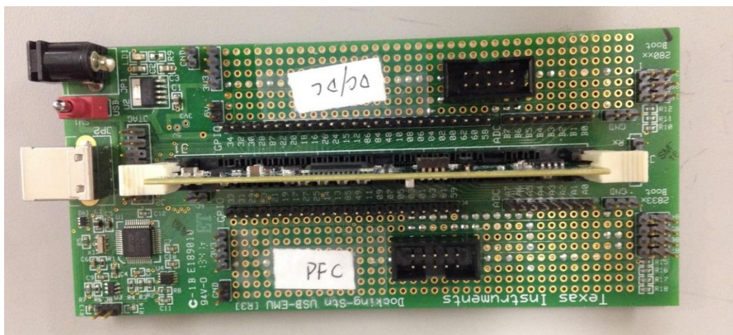
Fig. 6.35. Designed ac/dc SEPIC PFC converter prototype.
