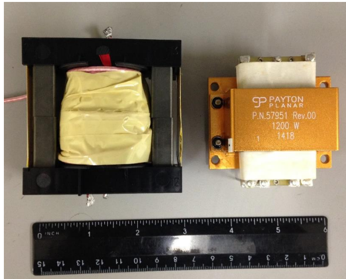
Fig. 7.3. LLC transformers switched at 200 kHz, and 1 MHz (from the left to the right).
