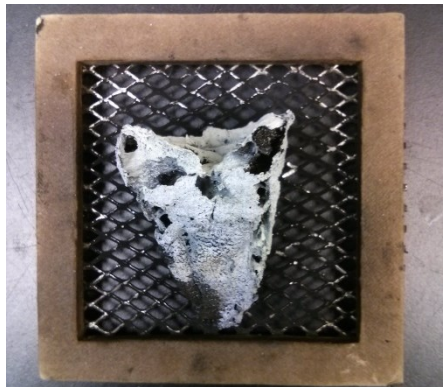
Figure 8.5 Char residues after gasification experiments for Kydex at 50 \text{ kW m}^{-2} .
