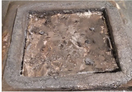
Figure 8.1 Char residues after gasification experiments for ABS at 50 \text{ kW m}^{-2} .
