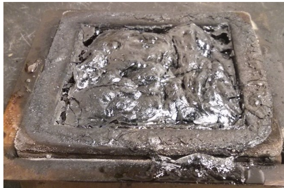
Figure 8.3 Char residues after gasification experiments for PET at 50 \text{ kW m}^{-2} .
