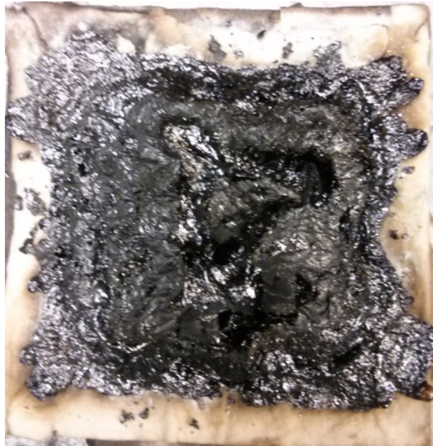
Figure 8.7 Char residues after gasification experiments for PEI at 50 kW m -2 .
