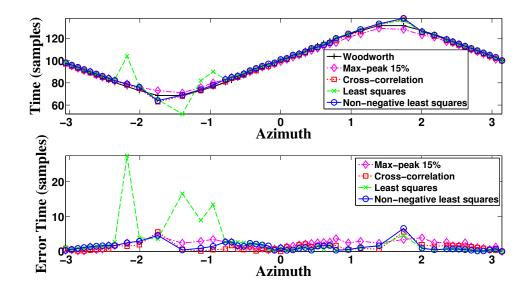
Figure 5.3: Horizontal plane ITD errors, computed over various methods (max-peak, cross-correlation, least squares, and NNLS), w.r.t. the Woodworth model [2] (ITD =  $a(\phi + \sin \phi)/c$  for the sphere radius a anthropometric parameter  $X_2/2$ , sound speed c, and azimuth  $\phi$  in radians) are shown.
