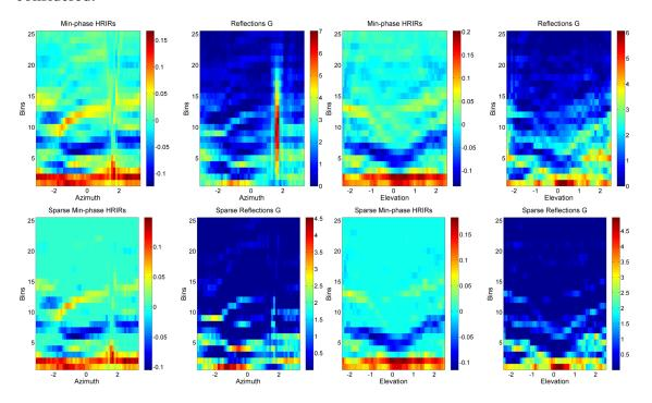
Figure 6.3: Top row: Slices of reflection filter matrix G trained without sparsity constraint; also, original HRIR after min-phase processing, time delay removing, and normalization. Bottow row: Slices of reflection filter matrix G trained with sparsity constraint applied ( $\lambda=10^{-3}$ ); also, HRTR reconstructed from it.
