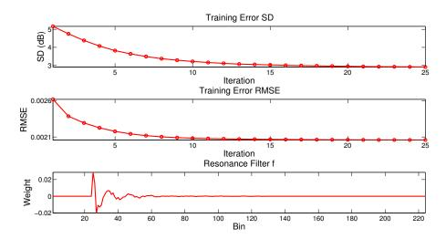
Figure 6.2: RMSE / SD error progress over 25 algorithm iterations.
