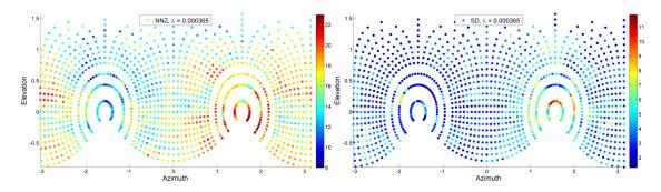
Figure 6.5: A map of NNZE and SD error over the full spherical coordinate range for left-ear HRIR data. Note smaller NNZE / SD values on ipsilateral side.
