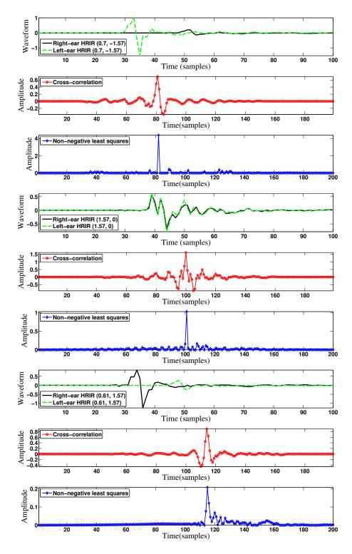
Figure 5.4: Cross-correlation and NNLS solutions for HRIR pairs on the azimuth plane (negative, zero, and positive time-delays centered at 100 time-samples) are shown.
