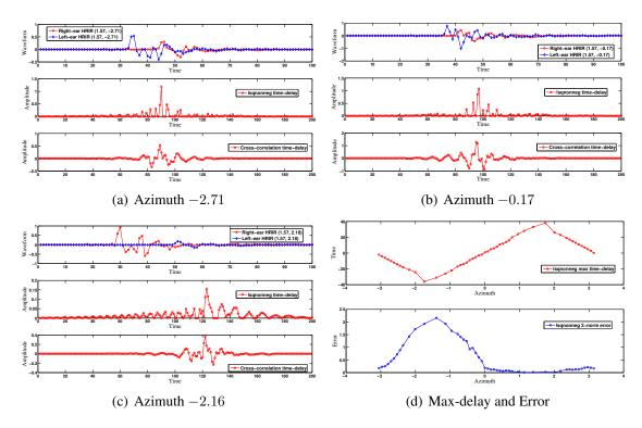
Figure 5.2: ITD of left and right ear CIPIC HRIRs on the Azimuth plane for subject 3 are shown. The x-axis represents integer time-bins.
