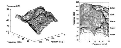
Figure 1.2: Log-magnitude HRTFs are smooth along spatial and frequency domains (horizontal and vertical plane directions are shown).
