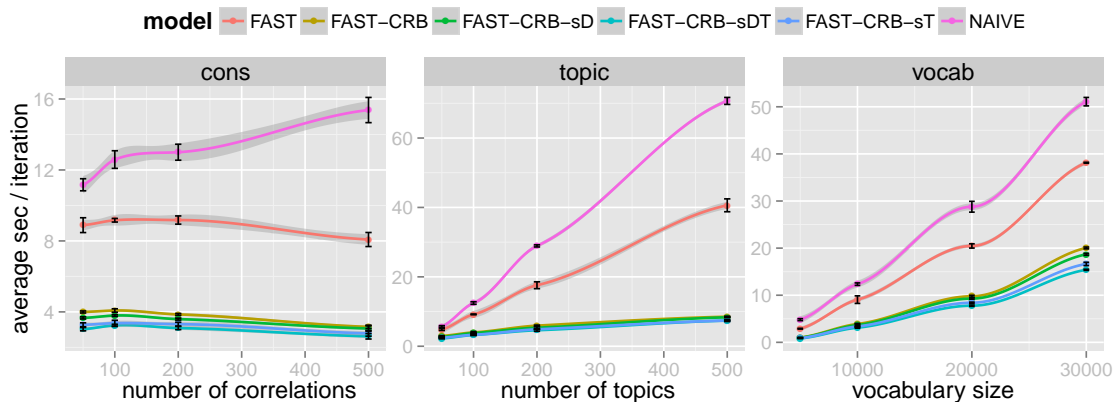
Figure 3.5: New York Times’ average running time per iteration (Sec) over 100 iterations, averaged over 5 seeds. Experiments begin with 100 topics, 100 correlations, vocab size 10000 and then vary one dimension: number of correlations (left), number of topics (middle), and vocabulary size (right).
