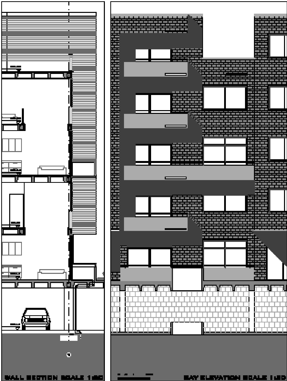
Figure 78. Wall section and bay elevation showing concrete frame construction and brick masonry [author] Figure 78. Wall section and bay elevation showing concrete frame construction and brick masonry [author]
