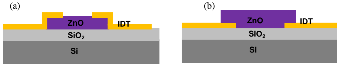
Figure 2.12: Cross sectional views of (a) traditional SAW sensor and (b) inverted SAW sensor for PLD ZnO deposition
