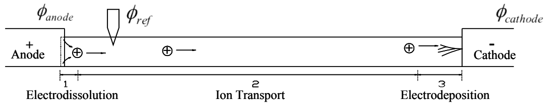
Figure 2: The ECM process that occurred on the surface of the comb structure.
