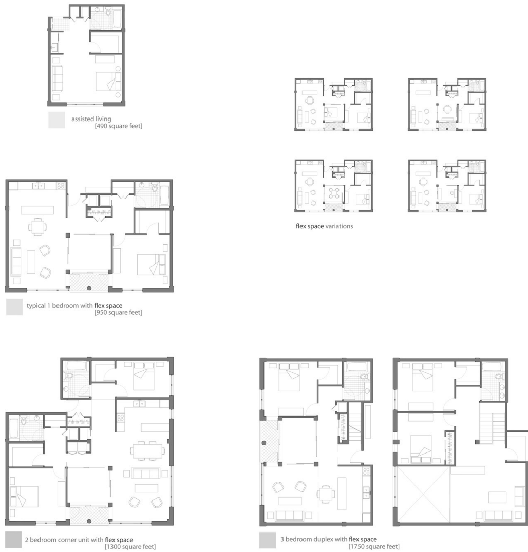
Figure 97. Typical Unit Plans: shows flex spaces and the ability to accommodate various family types. (Illustrated by author)
