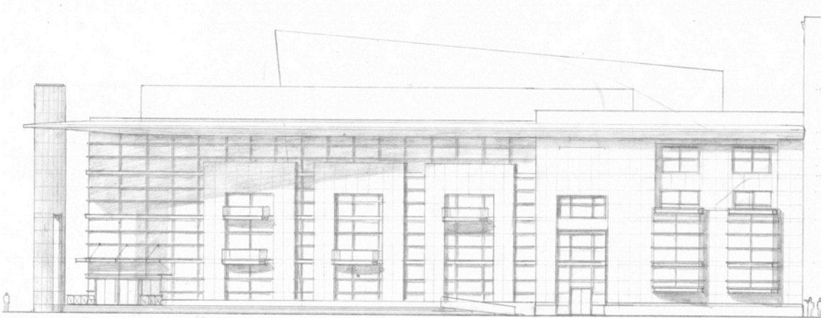
Figure 167 Study IX attempts to break down a large curtain wall with repeating balcony bays
