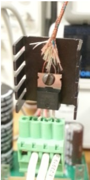
Figure 5 – Thermocouple fastened to the device's heat sink using a screw and an aluminum heat spreader.
